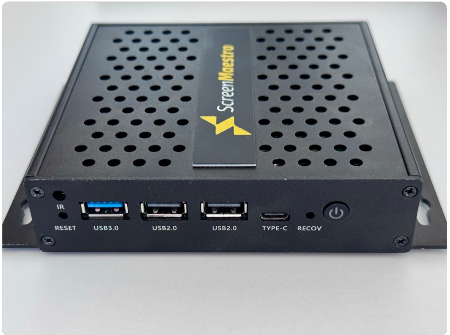
SCM Box front — USB ports for splitter power are here.
